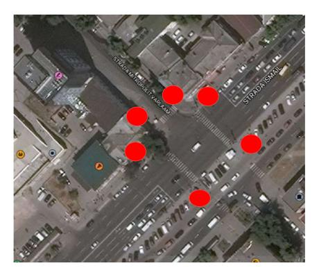
Figure 9. Six acoustic traffic lights were installed at the Ismail-Varlaam intersection
